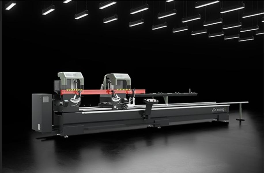
Electronic twin-head cutting-off machine with automatic traverse of the moving cutting head powered by brushless motor with numerical control system. Pneumatic control of the angular setting in three fixed positions 90°, 45° and 22°30' (external) or with mechanic system for manual adjustment of intermediate angles. Hydro-pneumatic blade feed.
