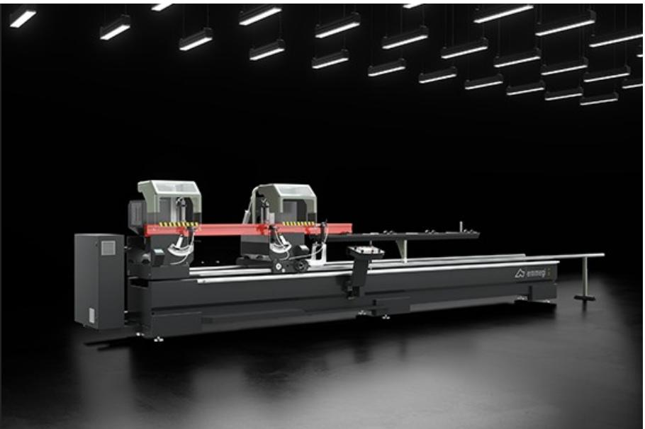
Electronic twin-head cutting-off machine with automatic traverse of the moving cutting head powered by brushless motor with numerical control system. Pneumatic control of the angular setting in three fixed positions 90°, 45° and 22°30' (external) or with mechanic system for manual adjustment of intermediate angles. Hydro-pneumatic blade feed.
