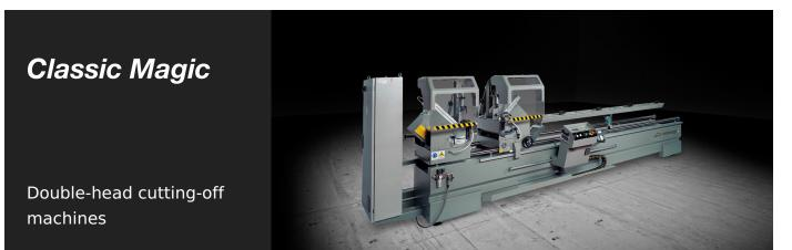
Electronic double-head cutting off machine with automatic movement of the mobile head through a C.C. motor controlled by numerical control. Pneumatic management of all angles up to 22°30′ (external). 450 and 500 mm-blade. Available with a useful cut of 4, 5, 6 m in length.
