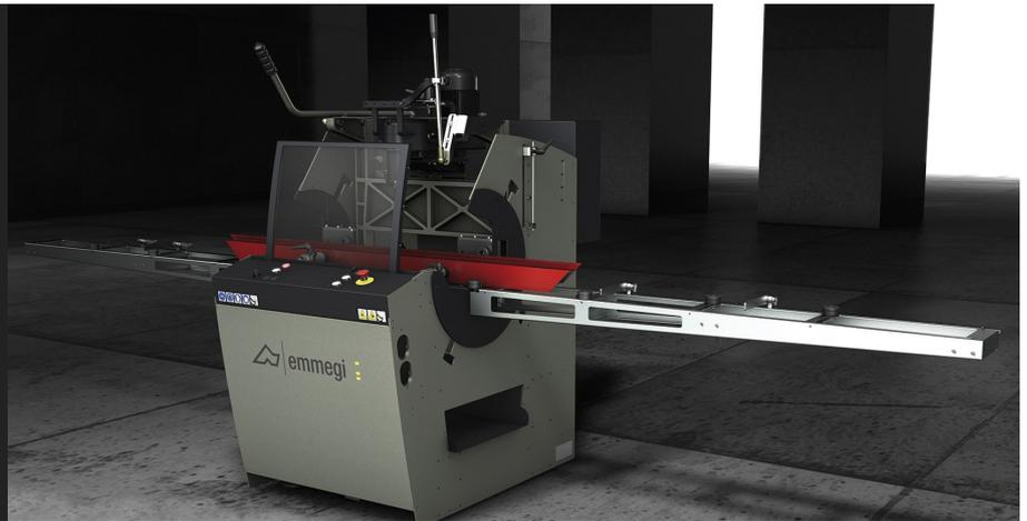
Manually controlled single head copy router with pneumatic clamping and traverse of the head with indirect lever. Tool rotation speed editable with electronic inverter to allow the machining of steel up to 2 mm, and to improve the quality of milling and tool life. Ability to run through machining of aluminum without turning the workpiece. Scratch-proof. Manually controlled stylus.
