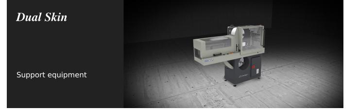
Machine for application of protective film on aluminium profiles. The profile is fed automatically via motorized rolls while the perfect adhesion of the film to the profile is ensured by pressure rolls. An optional additional kit allows applying the film simultaneously also on a third face.
