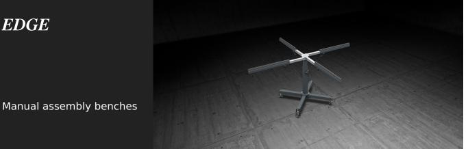
The bench is suitable for accessories and gaskets assembly. It can rotate on a central fulcrum and can be adjustable in length, thus allowing the frame rotation.
