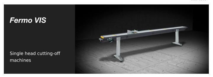
Stop gauge system with profile support, positioning of the stop via handwheel and reading of position on the digital readout. Tolerance on positioning  $\pm$  0.5 mm.
