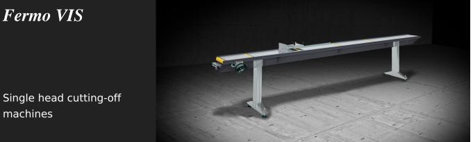
Stop gauge system with profile support, positioning of the stop via handwheel and reading of position on the digital readout.
