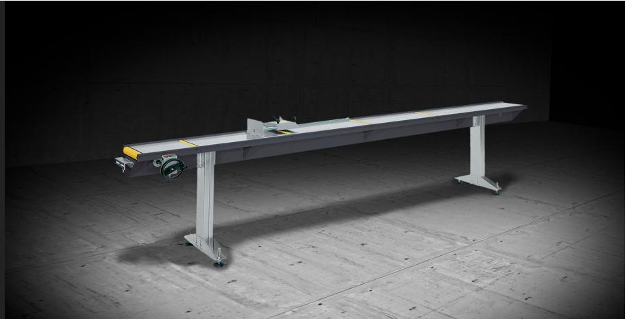
Stop gauge system with profile support, positioning of the stop via handwheel and reading of position on the digital readout.
