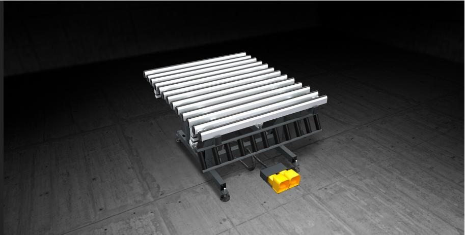
Sash and casement assembly bench. Tilting table from 0° (horizontal) to 85°, with pneumatic exchange between the soft PVC resting surface (for assembly operations) and the anti-friction hard PVC resting surface (for handling operations). The roller conveyor can be manually tilted and it is adjustable in height (from 170 to 460 mm) independently from the work table height. The work table height is adjustable from 895 to 965 mm and the mounting feet are complete with holes for floor anchoring.
