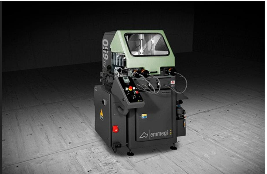
Single-head, rising blade cutting-off machine for large sections. Designed for cutting at 90° only.
