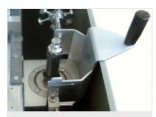
Quick tool change Quick milling tool change, manually controlled by a lever.
