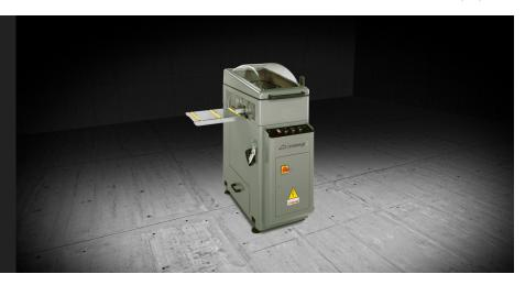
Horizontal end milling machine with manual feed. Milling of intermediate angles, +45° / 90° / -45°. High speed of tool rotation for improved quality machining on painted profiles and at intermediate angles. Quick cutter change with pneumatic control. Scratch-proof work table. Fully guarded work zone with high internal visibility
