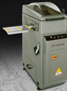
Horizontal end milling machine with manual feed. Milling of intermediate angles,  $+45^\circ / 90^\circ / -45^\circ$ . High speed of tool rotation for improved quality machining on painted profiles and at intermediate angles. Quick cutter change with pneumatic control. Scratch-proof work table. Fully guarded work zone with high internal visibility
