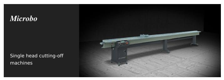
Stop gauge and profile support system, driven by DC motor, complete with electronic read-out through encoder.
