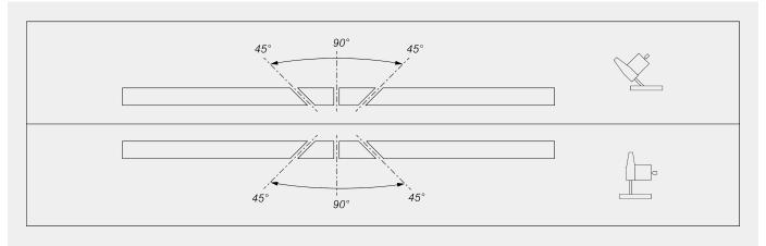
Mechanical adjustment of intermediate angles
