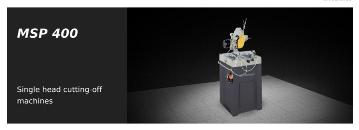
Single-head, descending blade cutting-off machine with left loading side, rotation of the cutting head to 45° (left and right) and manual tilting by 45° referred to the horizontal axis.
