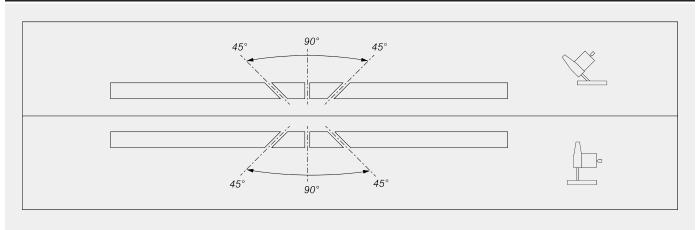
Mechanical adjustment of intermediate angles
