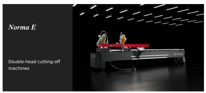
Double head cutting-off machine with manual movement of the mobile head and position detection by means of an absolute magnetic band. The rotation of the cutting units on the vertical axis (45° to the left and right) and the inclination on the horizontal axis (45° internal), with manual adjustment, allow combined cuts even at intermediate angles.
