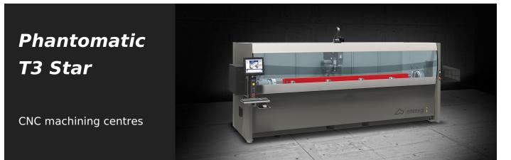
Machining centre CNC with 4 controlled axes, used for working bars of aluminium, PVC, light alloys in general and steel pieces up to 3 mm. It has a 4 tool magazine, with the possibility of hosting 2 angular units and one milling disc. The presence of the rotary work table (CN axis) allows machining at any angle from - 90° to + 90° and on the two heads with a double output angle machining head, with the table at 0°. All CNC axes are absolute and do not require resetting upon machine restart.
