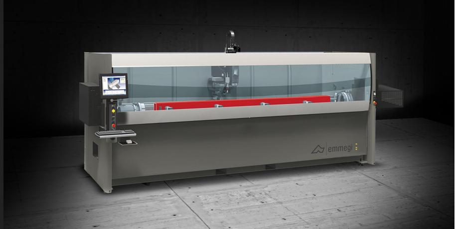
Machining centre CNC with 4 controlled axes, used for working bars of aluminium, PVC, light alloys in general and steel pieces up to 3 mm. It has a 4 tool magazine, with the possibility of hosting 2 angular units and one milling disc. The presence of the rotary work table (CN axis) allows machining at any angle from - 90° to + 90° and on the two heads with a double output angle machining head, with the table at 0°. All CNC axes are absolute and do not require resetting upon machine restart.
