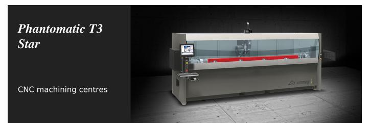
Machining centre CNC with 4 controlled axes, used for working bars of aluminium, PVC, light alloys in general and steel pieces up to 3 mm. It has a 4 tool magazine, with the possibility of hosting 2 angular units and one milling disc. The presence of the rotary work table (CN axis) allows machining at any angle from - 90° to + 90° and on the two heads with a double output angle machining head, with the table at 0°. All CNC axes are absolute and do not require resetting upon machine restart.
