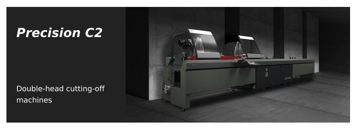
Electronic twin-head cutting-off machine with frontal blade Electronic twin-head cutting-off machine with the moving cutting head powered by brushless motor with numerical control system. Pneumatic control of the angular setting from 90° to 22°30′ (external) with mechanic adjustment of intermediate angles. Hydropneumatic blade feed. Available in two versions with 4000 and 5000 mm cutting length.
