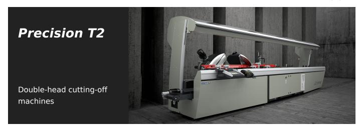
Double-head cutting-off machine with 3 controlled axes for aluminium, PVC and light alloys with automatic movement of the mobile head and electronic management of all 45° (internal) to 15° (external) angles, with a precision, within each degree, of 280 positions. In the basic version blade advancement is driven by a couple of hydro-pneumatic cylinders. 550mm-blade. Available with a useful cut of 5 m or 6 m in length.
