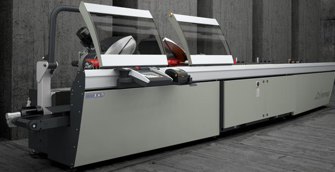
Twin-head cutting-off machine with 3 controlled axes, automatic traverse of the moving cutting head and electronic control of every angular setting from 45° (internal) to 15° (external) with accuracy of 280 places on each degree. The blade feed is controlled by two hydro-pneumatic cylinders.
