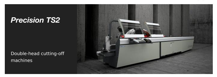
Twin-head cutting-off machine with 3 controlled axes, automatic traverse of the moving cutting head and electronic control of every angular setting from 45° (internal) to 15° (external) with accuracy of 280 places on each degree. The blade feed is controlled by two hydro-pneumatic cylinders.
