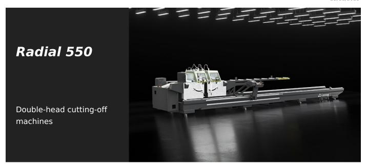
Electronic twin-head cutting-off machine with radial blade movement, automatic traverse of the moving head on recirculating ball bearings by rack and pinion system; tilting inwards up to 30°, designed for cutting large profiles. The blade feed is controlled by two hydro-pneumatic cylinders.
