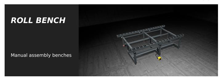
Large size modular bench for assembly and in-line handling of curtain wall frames. It is provided with two roller tracks covered with soft PVC sheathing; the distance between the two tracks is adjustable according to the width of the curtain wall section. A pneumatically operated system allows clamping the rollers during the work phases.
