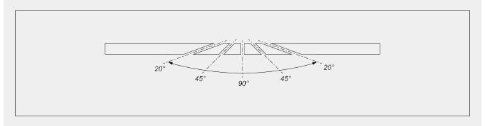
Mechanical adjustment of intermediate angles
