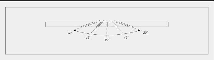
Mechanical adjustment of intermediate angles
