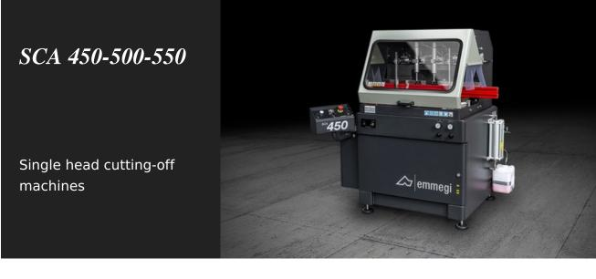
Single-head, rising blade cutting-off machine, with left loading side, able to perform cuts from 20° left to 20° right and intermediate angles.
