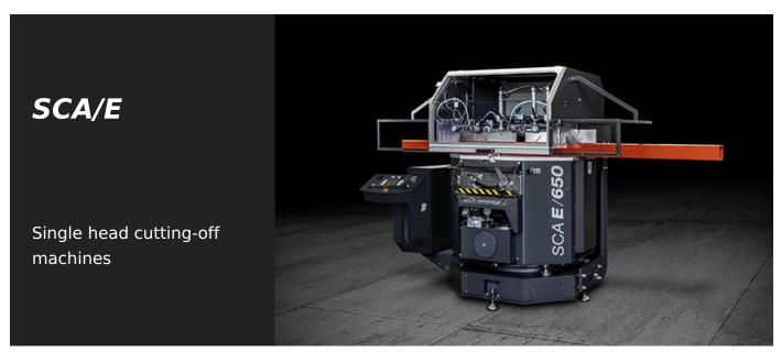
Single-head, rising blade cutting-off machine, with N/C automatic rotation of the vertical axis through brushless motor and contemporaneous hydraulic tilting of the horizontal axis. Cutting with angular settings from 90° to 22°30′ (left and right) on the vertical axis and from 90° to 35° (right only) on the horizontal axis.
