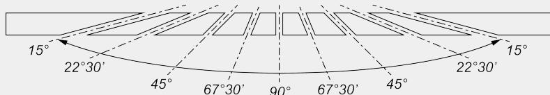
Mechanical adjustment of intermediate angles
