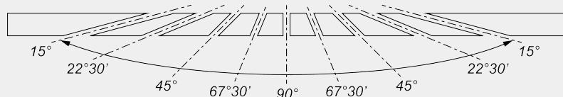
Mechanical adjustment of intermediate angles
