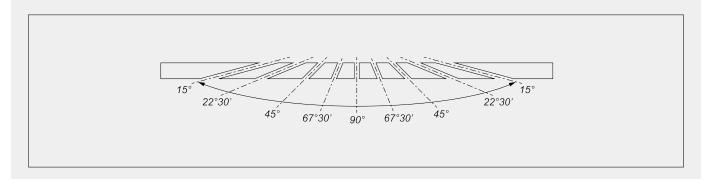
Mechanical adjustment of intermediate angles
