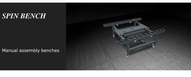
Modular bench for assembly and in-line handling of curtain wall frames. It is provided with two roller tracks covered with soft PVC sheathing; the distance between the two tracks is adjustable according to the width of the curtain wall section. A pneumatically operated system allows clamping the rollers during the work phases. The entire bench can be rotated by 360° in order to facilitate the assembly and sealing of the curtain wall; the angular position is clamped pneumatically.
