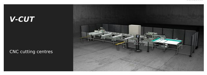
Fully automatic CNC cutting centre with 3 controlled axes, designed for cutting profiles of aluminium, PVC, or light alloys in general. Starting off from the extruded barstock, V-CUT carries out the loading, cutting and unloading of predefined and optimized cutting lists automatically. It is able to perform cuts from 45° to 135° or from 22°30′ to 157°30′.
