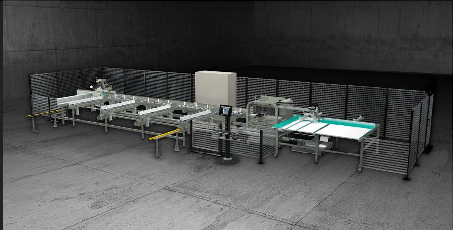
Fully automatic CNC cutting centre with 3 controlled axes, designed for cutting profiles of aluminium, PVC, or light alloys in general. Starting off from the extruded barstock, V-CUT carries out the loading, cutting and unloading of predefined and optimized cutting lists automatically. It is able to perform cuts from 45° to 135° or from 22°30' to 157°30'.
