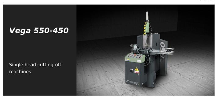
Single-head cutting-off machine with horizontal blade feed and left loading side, pneumatic double side tilting of the cutting head in fixed positions: 45° to the left, 90°, 45° and 22°30′ to the right. A special positive stop also allows cutting at intermediate angles.
