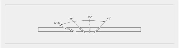
Mechanical adjustment of intermediate angles
