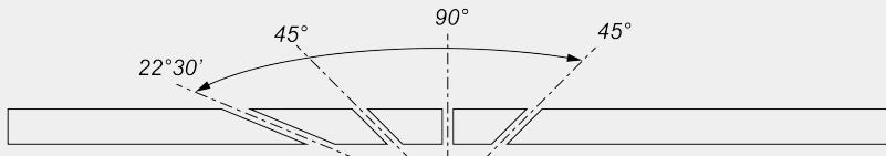
Mechanical adjustment of intermediate angles
