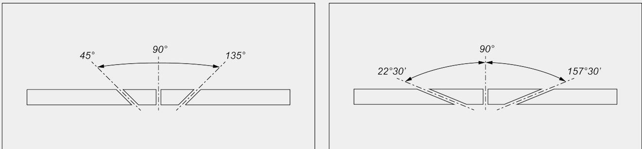
Electronic adjustment of intermediate angles
