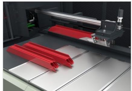
**Extraction system for machined workpiece**
