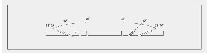
Mechanical adjustment of intermediate angles
