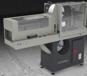
Machine for application of protective film on aluminium profiles. The profile is fed automatically via motorized rolls while the perfect adhesion of the film to the profile is ensured by pressure rolls. An optional additional kit allows applying the film simultaneously also on a third face.
