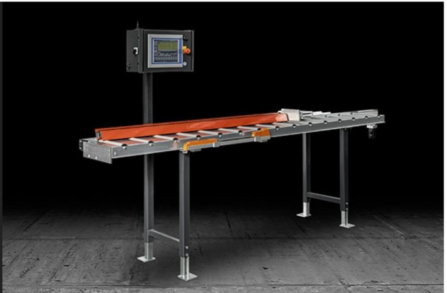
Stop gauge and profile support system with movement of the stop on CN axis and electronic read-out by absolute magnetic band. Equipped with an electronic measurement system that allows to save data on internal memory or transferred in real time to a PC or to the control unit of a miter saw via Bluetooth. It allows machining with high accuracy and repeatability of positioning.
