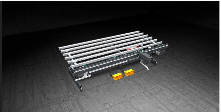
Assembly bench for fitting perimetral band-cut hardware on aluminium, wood and PVC sashes. A system of drop-away vices grips the sash. The bench is equipped with an automatic feeding screwing system and optionally with a system for hardware cutting and measuring with hydro-pneumatic shears.
