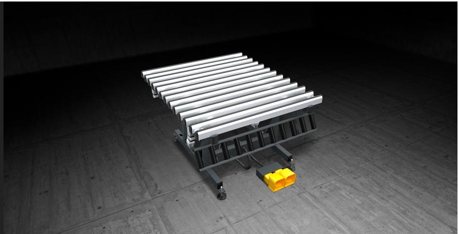
Sash and casement assembly bench. Tilting table from 0° (horizontal) to 85°, with pneumatic exchange between the soft PVC resting surface (for assembly operations) and the anti-friction hard PVC resting surface (for handling operations). The roller conveyor can be manually tilted and it is adjustable in height (from 170 to 460 mm) independently from the work table height. The work table height is adjustable from 895 to 965 mm and the mounting feet are complete with holes for floor anchoring.
