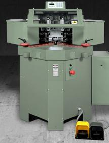
The machine has two special operating heads equipped with masses in which the 2 knives are adjustable on all crimping positions. The knives move and are adjustable on the Y axis (along the profile), on the Z axis (top-bottom) and on the X axis (along the crimping direction). These conditions prevent the replacement of tools on the machine regardless of the different types of profiles. In this way, the times and costs of placing are reduced.
