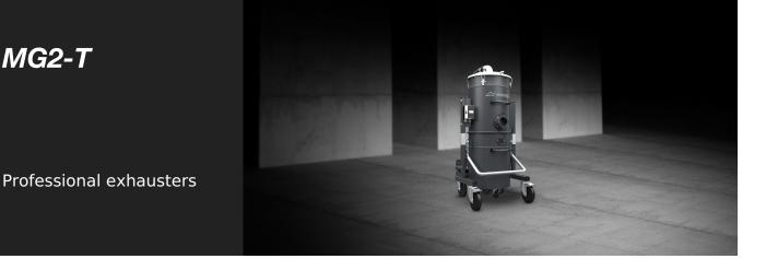
Extraction system for aluminium and PVC swarf with single suction nozzle, designed for cleaning machines and the work environment or extract swarf from work units that require high vacuum values. The use of a high-depression side duct turbine makes it suitable for various extraction requirements. Equipped with an anti-static filter, this is a wheel-mounted, quick-release, automatic vibrating filter and collection tank cleaning system, to dispose of exhausted material easily and quickly.
