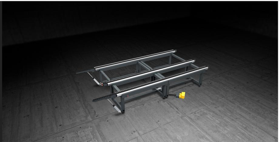
Large size and extendible modular bench for assembling of windows and curtain wall frames. It features 3 distinct work tables: one of soft PVC for assembly operations, one of anti-friction hard PVC for the rotation and a roller conveyor for in-line movements.
