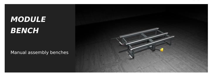
Large size and extendible modular bench for assembling of windows and curtain wall frames. It features 3 distinct work tables: one of soft PVC for assembly operations, one of anti-friction hard PVC for the rotation and a roller conveyor for inline movements.
