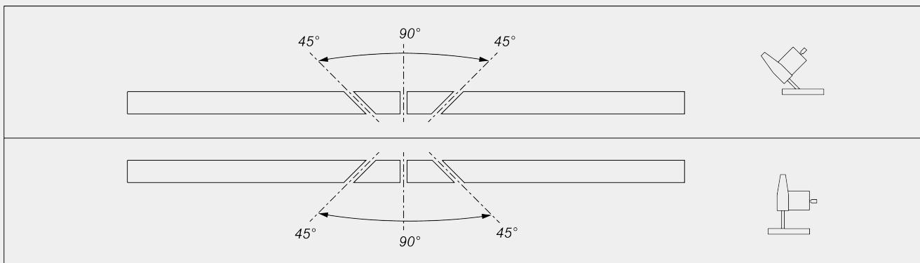
Mechanical adjustment of intermediate angles
