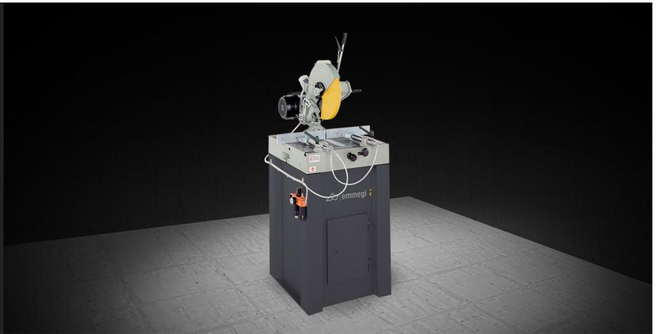
Single-head, descending blade cutting-off machine with left loading side, rotation of the cutting head to 45° (left and right) and manual tilting by 45° referred to the horizontal axis.
