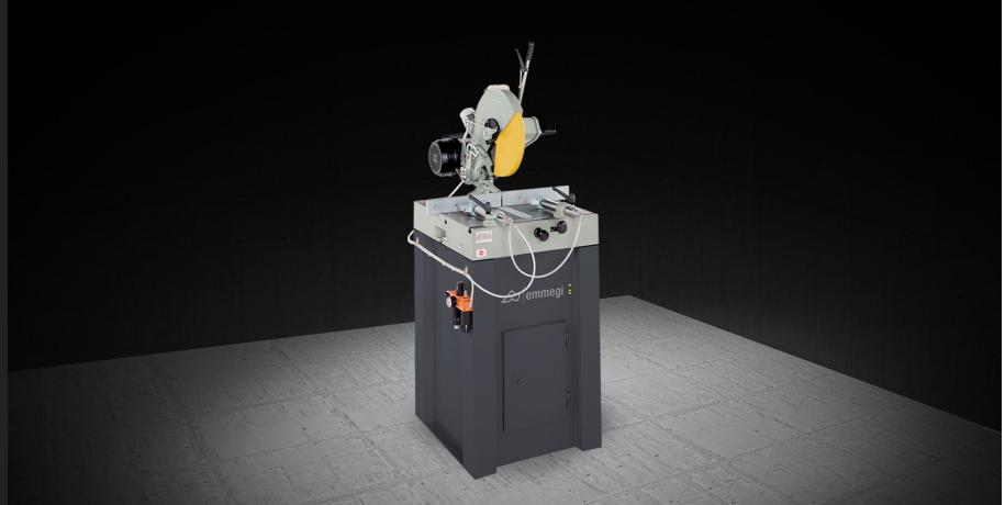
Single-head, descending blade cutting-off machine with left loading side, rotation of the cutting head to 45° (left and right) and manual tilting by 45° referred to the horizontal axis.
