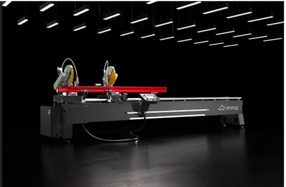
Double head cutting-off machine with manual movement of the mobile head and position detection by means of an absolute magnetic band. The rotation of the cutting units on the vertical axis ( $45^\circ$  to the left and right) and the inclination on the horizontal axis ( $45^\circ$  internal), with manual adjustment, allow combined cuts even at intermediate angles.
