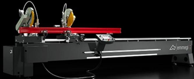
Double head cutting-off machine with manual movement of the mobile head and position detection by means of an absolute magnetic band. The rotation of the cutting units on the vertical axis (45° to the left and right) and the inclination on the horizontal axis (45° internal), with manual adjustment, allow combined cuts even at intermediate angles.
