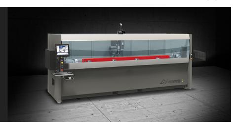
Machining centre CNC with 4 controlled axes, used for working bars of aluminium, PVC, light alloys in general and steel pieces up to 3 mm. It has a 4 tool magazine, with the possibility of hosting 2 angular units and one milling disc. The presence of the rotary work table (CN axis) allows machining at any angle from - 90° to + 90° and on the two heads with a double output angle machining head, with the table at 0°. All CNC axes are absolute and do not require resetting upon machine restart.
