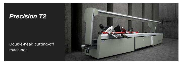
Double-head cutting-off machine with 3 controlled axes for aluminium, PVC and light alloys with automatic movement of the mobile head and electronic management of all 45° (internal) to 15° (external) angles, with a precision, within each degree, of 280 positions. In the basic version blade advancement is driven by a couple of hydro-pneumatic cylinders. 550mm-blade. Available with a useful cut of 5 m or 6 m in length.
