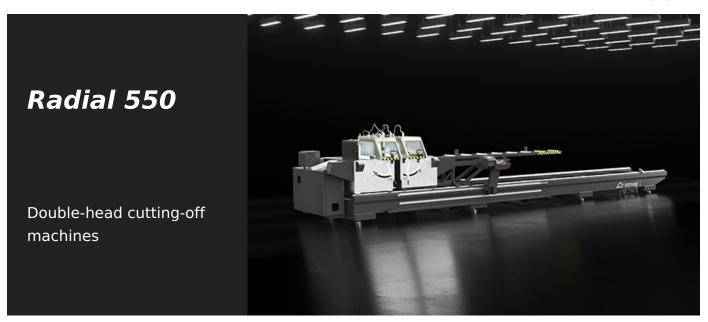
Electronic twin-head cutting-off machine with radial blade movement, automatic traverse of the moving head on recirculating ball bearings by rack and pinion system; tilting inwards up to 30°, designed for cutting large profiles. The blade feed is controled by two hydro-pneumatic cylinders.
