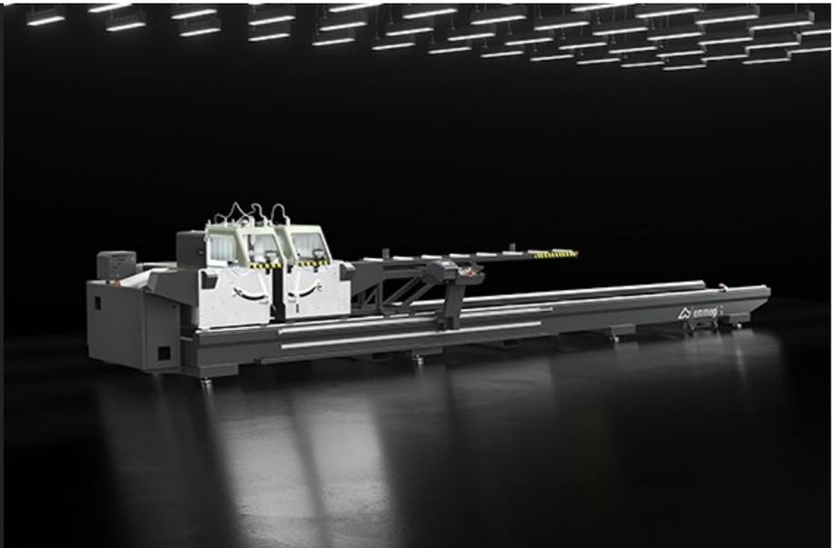
Electronic twin-head cutting-off machine with radial blade movement, automatic traverse of the moving head on recirculating ball bearings by rack and pinion system; tilting inwards up to 30°, designed for cutting large profiles. The blade feed is controlled by two hydro-pneumatic cylinders.
