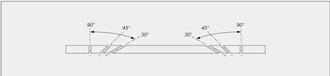
Electronic adjustment of intermediate angles
