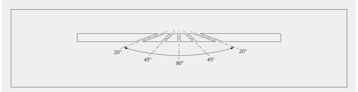
Mechanical adjustment of intermediate angles
