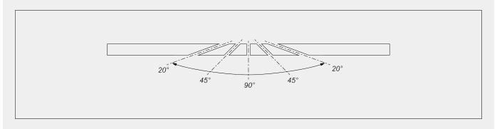
Mechanical adjustment of intermediate angles
