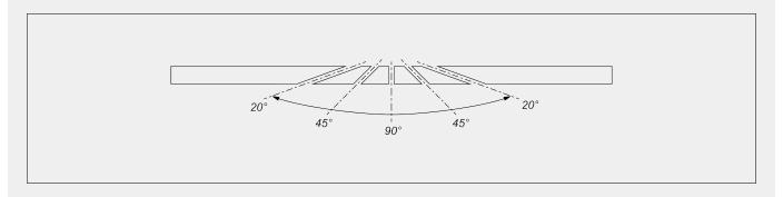
Mechanical adjustment of intermediate angles
