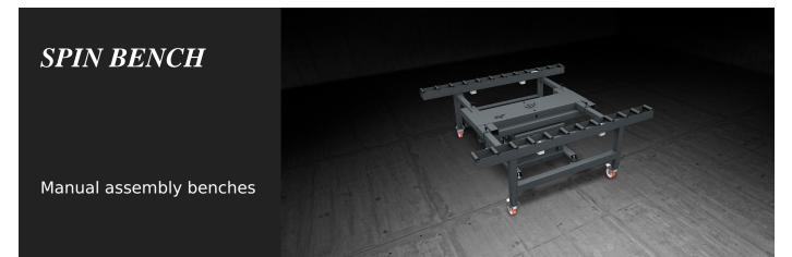
Modular bench for assembly and in-line handling of curtain wall frames. It is provided with two roller tracks covered with soft PVC sheathing; the distance between the two tracks is adjustable according to the width of the curtain wall section. A pneumatically operated system allows clamping the rollers during the work phases. The entire bench can be rotated by 360° in order to facilitate the assembly and sealing of the curtain wall; the angular position is clamped pneumatically.
