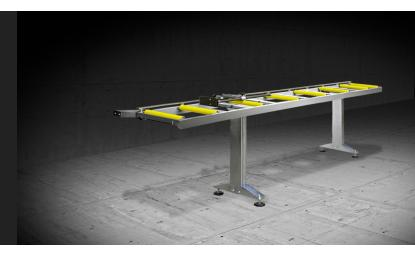
Tubular steel construction with adjustable mounting feet and PVC covered steel rolls. In the version with rolls size 240 mm, roller conveyor length is 3.500 mm; with rolls size 440 mm, roller conveyor length is 4.000 mm.
