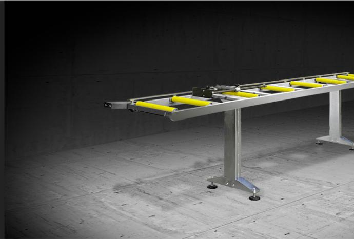
Tubular steel construction with adjustable mounting feet and PVC covered steel rolls. In the version with rolls size 240 mm, roller conveyor length is 3.500 mm; with rolls size 440 mm, roller conveyor length is 4.000 mm.
