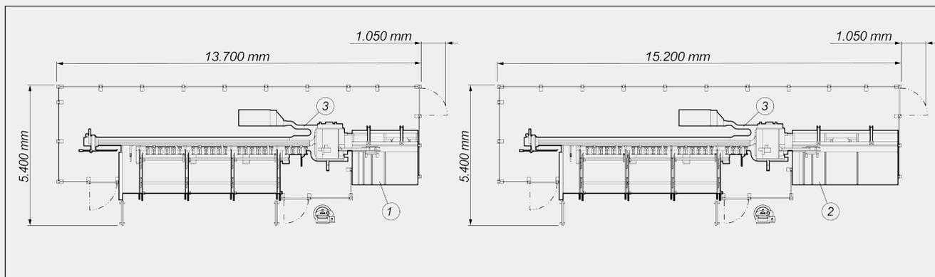
1. Storage unit for workpieces up to 2500 mm (standard)
