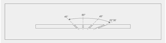
Mechanical adjustment of intermediate angles
