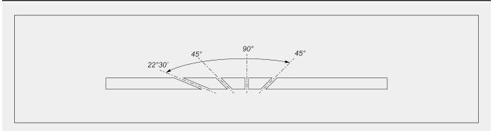
Mechanical adjustment of intermediate angles
