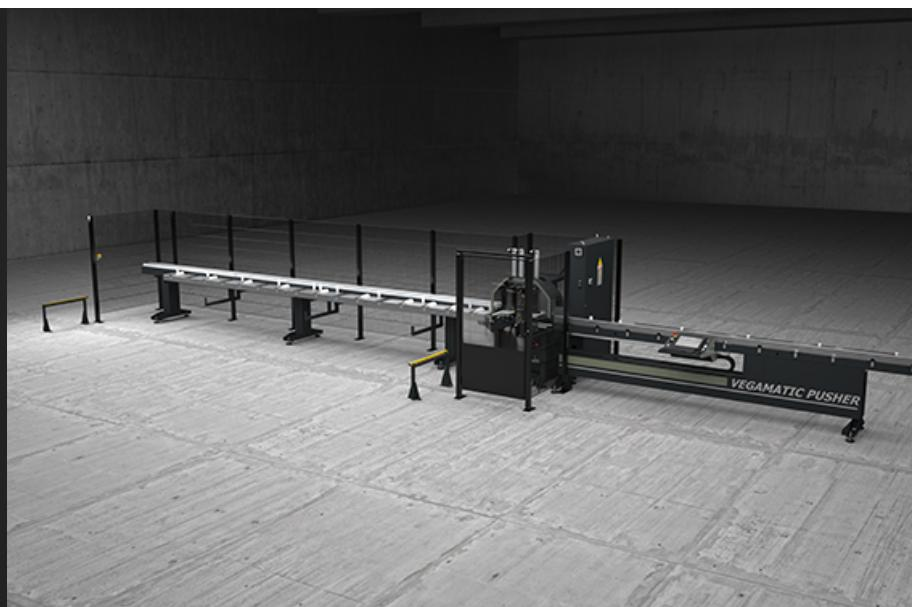
A semiautomatic version cutting centre with 2 controlled axes, manual loading/unloading on opposite sides of the machine, with front CNC blade, dedicated to cutting Aluminium and PVC profiles and light alloys in general. It performs predefined and optimised cutting lists in automatic. Designed to execute cutting at angles ranging from 45° to 135° or from 22°30' to 157°30'. Configurable with horizontal or vertical drilling units that can be personalised for specific automatic machining.
