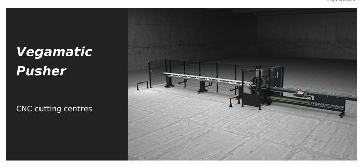
A semiautomatic version cutting centre with 2 controlled axes, manual loading/unloading on opposite sides of the machine, with front CNC blade, dedicated to cutting Aluminium and PVC profiles and light alloys in general. It performs predefined and optimised cutting lists in automatic. Designed to execute cutting at angles ranging from 45° to 135° or from 22°30' to 157°30'. Configurable with horizontal or vertical drilling units that can be personalised for specific automatic machining.
