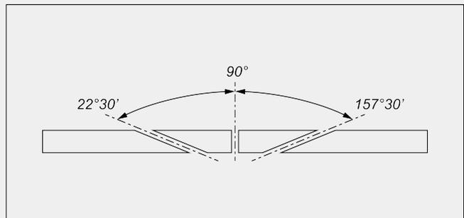
Electronic adjustment of intermediate angles
