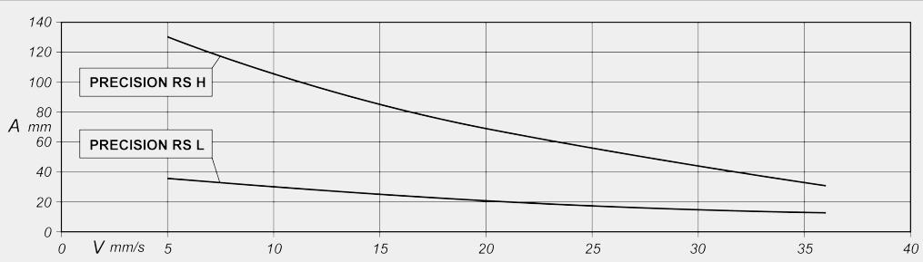
A = 接触弧 (mm) V = 刀片进给速度 (mm/s)
