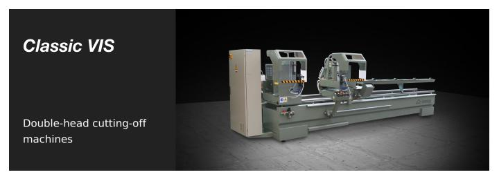
Double head cutting-off machine with manual movement of the mobile head and parameter reading through digital display screen. Outward pneumatic tilting of the head up to 45° or 22°30′ depending on the model. 450 and 500 mm-blade. Available with a useful cut of 4, 5, 6 m in length.
